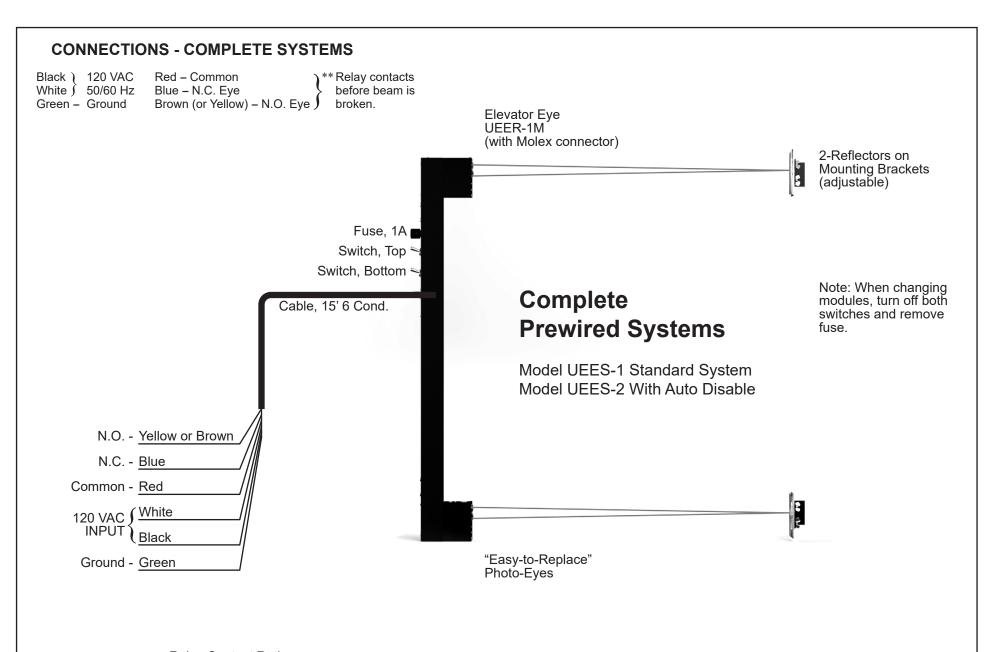
Relay Contact Rating: AC 250V = 2 AMP DC 30V+ 3 AMP
